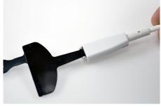
Slide the cover on the cable over the flex sensor.
