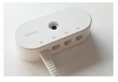
Plug the micro USB cable into a previously installed S2865 Power/ Alarm box or Zips Alarm Unit.
