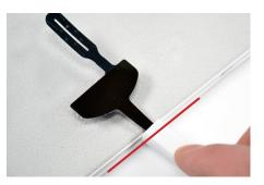
On the felted side of the backcover/kickstand, carefully align the cover of the flex sensor connector cable with the edge, in the location determined in Step 16.
