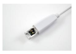
Slide the cover on the flex sensor connector cable back to reveal the contacts.
