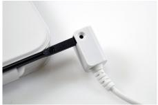
Insert the bar into the square opening in the sensor. Ensure that the screw holes on the bar and sensor are aligned.
