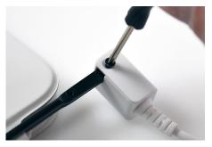
Use the provided screwdriver to tighten the screw, securing the sensor to the bar.
