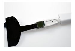
Place the flex sensor appropriate for your installation into the flex sensor connector cable.
