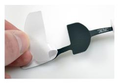
Peel the liner from the Side Mount flex sensor.
