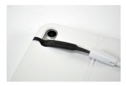
Place the back cover/kickstand onto the back of the tablet. Slide the flex sensor over so that it will not block the cover.
