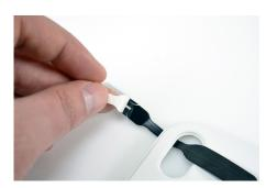
Peel the liner from the flex sensor.
