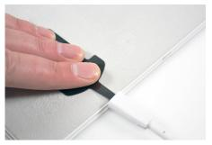
Press the flex sensor against the felted surface for at least 10 seconds.
