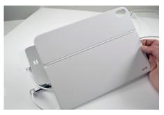
Remove the back cover/kickstand from the tablet.
