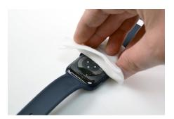
Use a provided alcohol wipe to clean the bottom and sides of the wearable. Allow it to dry completely.
