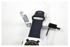
With the wearable facing down, place the back band into the band clamp as shown.
