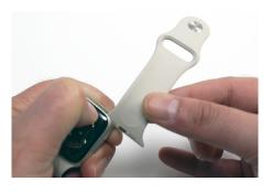
Remove the buckle band from the device.
