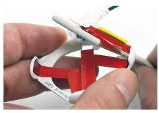
Insert the band through the gap on the back side of the tray sensor.
