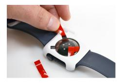
Flip the wearable over and pull all of the red tabs out through the opening in the bottom of the tray sensor.
