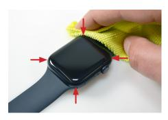
Carefully rub the polish onto the corners of the wearable for 15-20 seconds.
