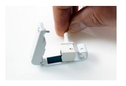
Slide the sensor end from the existing band clamp.
