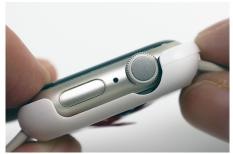
Ensure that the dial fits into the cut out on the tray sensor.
