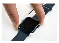
Press all adhesives on the tray sensor against the wearable for at least 10 seconds.
