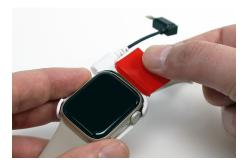
Place the device into the tray sensor. Pull the red tab to expose the upper bridge adhesive.
