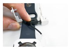
Plug the sensor on the flex tray into the sensor end of the stand.
