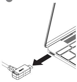
Unplug the OEM power supply from the port on the sensor cable. Note: The sensor is now ready to be reinstalled. Consult the installation guide for more information.
