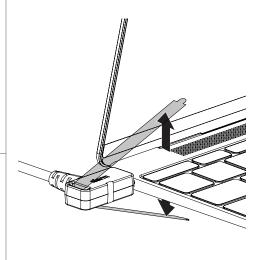
Use an alcohol wipe to remove any adhesive residue on the device and sensor.
