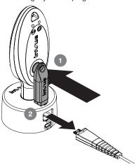
If using the S2865 system, place the charged and coded OneKEY onto the Remote IR Dot connected to the system and press the button. Remove the sensor from the S2865 Alarm/ Power Box.
