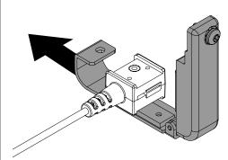
Slide the large band clamp onto the sensor. Proceed with the installation as normal.
