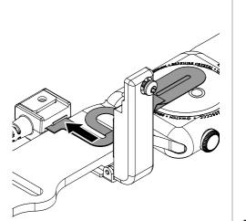
Adjust the wearable so that the area between the 2 white lines on the flex sensor (the shaded area in the below image) will sit over the "hinge" area (the area where the band connects to the watch body) of the wearable.
