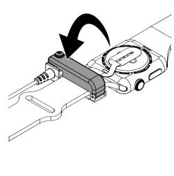
Press down on the band clamp and use a TT8 bit to tighten the screw in the band clamp. Do NOT overtighten.
