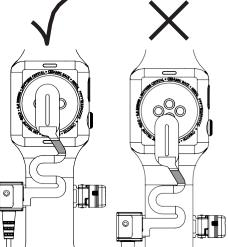
Peel the liner from the adhesive 14d portion of the flex sensor.
