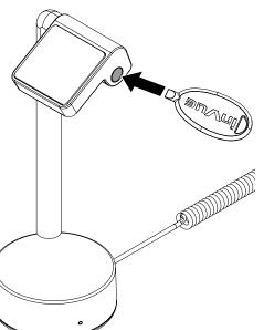
Remove the plug and screw from the side of the cradle.
