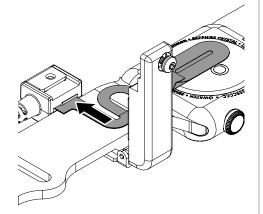
Adjust the wearable so that the area between the 2 white lines on the flex sensor (the shaded area in the below image) will sit over the "hinge" area (the area where the band connects to the watch body) of the wearable.
