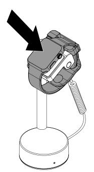
Plug the stand's power cable into a Zips alarm unit, S2865 power/alarm box, OnePOD aux port.
