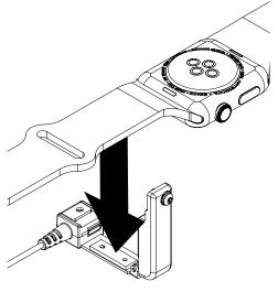
Plug the universal flex sensor into the port on the inside of the band clamp over the wearable.
