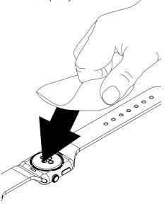
Use a TT8 bit to loosen the screw in the band clamp.
