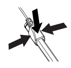
Plug the micro USB connector into a Zips! 2.0 alarm unit. The alarm unit will chirp.
