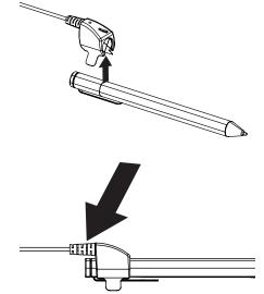
Pull the tabs on the adhesives and pinch the sensor against the stylus for at least 10 seconds.
