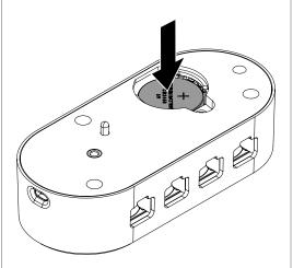
e Replace the battery door by first insert the small tab into the opening then pivoting the door down into the Alarm unit.
