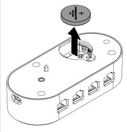
Insert the new CR2450, with the Positive Side (+) facing up, into the battery holder.
