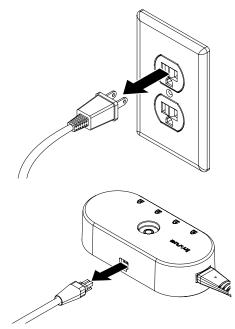
If used, unplug the remote IR dot from the Alarm Unit.
