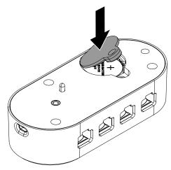
Insert and tighten the screw to secure the battery door.
