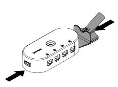
Peel the 2 old adhesives from the Alarm Unit.
