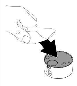
6a If the battery needs to be changed out, use a Philips head screwdriver to remove the 2 screws in the bottom of the Alarm Unit.
