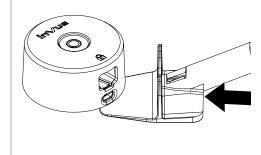
Peel the old adhesive from the Alarm Unit.
