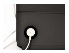
Place the secondary sensor onto the LSE plate in the predetermined position.
