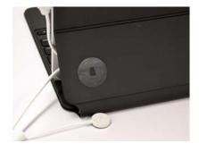
Remove one of the LSE plates from their backing and place it onto the keyboard cover with the narrower end facing up. Apply pressure for at least 10 seconds.
