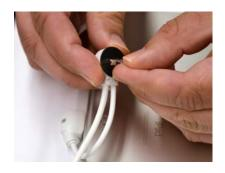
Peel the clear film from the adhseive sensor connected to the USB-C sensor.
