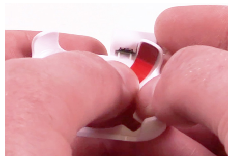
13 Carefully place the adhesive, with the pull tab facing towards the center of the sensor, into the corner.
