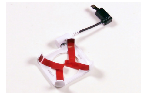
15 Repeat for the other 3 adhesives and corners. The sensor is now ready to be reinstalled.
