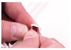
Carefully place the adhesive, with the pull tab facing towards the center of the sensor, into the corner.
