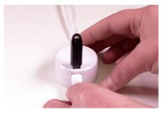
Place a DBG400 Magnet Key onto the lock icon on the Alarm Unit.
