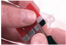
Carefully remove the small paper backing from one of the ADH2367 sensor replacement adhesives.
