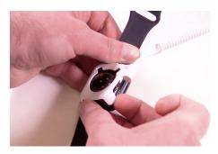
3 Carefully lift one corner of the sensor from the wearable.
