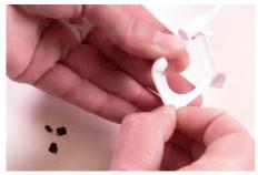
Remove any old adhesives from the corners of the sensor.
