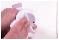
Use an alcohol wipe to clean any adhesive residue from the bottom of the stand. Allow it to dry completely.
