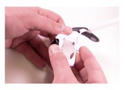
Lift the other corners away from the wearable and remove the sensor.
