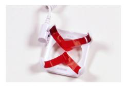
Repeat for the other 3 adhesives and corners. The sensor is now ready to be reinstalled.
