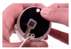
Remove one of the ADH2321 replacement adhesives from its backing and carefully align it with the bottom of the WS2 stand.
