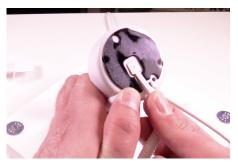
Remove the sensor from the bottom of the stand.
