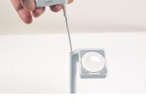
Lift the band clamp/sensor end from the stand.
