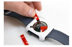
Flip the wearable over and pull the 4 red tabs out through the opening in the bottom of the tray sensor.
