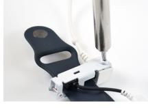
Use a TT8 bit to tighten the screw on the band clamp.
