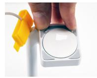
18 Place the aligner pad into the depression on the charging cradle and apply pressure for at least 10 seconds.
