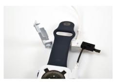
With the wearable facing down, place the back band into the band clamp as shown.
