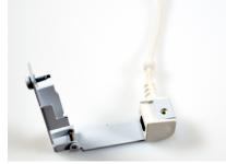
10 Slide the provided band clamp onto the sensor end so that the screw holes align.
