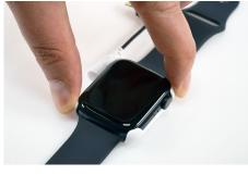
Press the 4 corners of the tray sensor against the wearable for at least 10 seconds.
