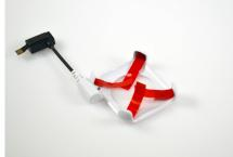
Ensure that the red pull tabs lay flat against the bottom of the tray sensor.
