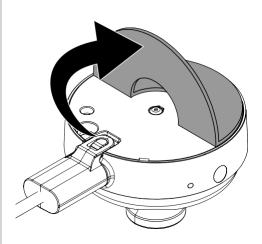
Use an alcohol wipe to clean any adhesive residue from the sensor.
