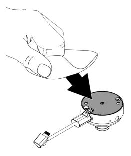
Remove one of the replacement adhesives (ADH2180) from it's backing and align it with the flat surface of the sensor. Smooth it into place for at least 10 seconds.
