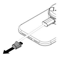
Insert the scraper removal tool (DNTX93) between the sensor and device. Carefully work the scraper tool back and forth to break the adhesive bond between the sensor and the device.
