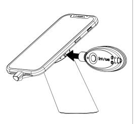
Remove the sensor and device from the stand. Place the magnet key (DBG400) into the depression on the sensor and push it inward to release the sensor cable. Pull the cable free.
