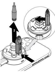
Unplug the power connector from the device
