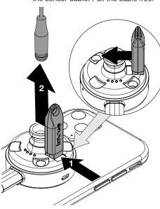
Unplug the power connector from the device.
