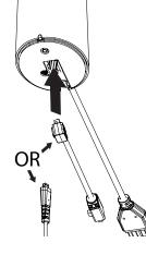
If routing power cable through fixture, drill a 19mm minimum, 22mm maximum hole in the fixture. **Do NOT mount the stand over a hole larger than 22mm.** If routing power cable above the fixture see step 2. Route power cable through hole or above fixture.
