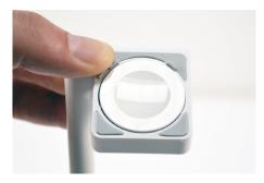
Place the aligner pad into the depression on the charging cradle and apply pressure for at least 10 seconds.
