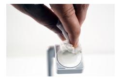
Use an alcohol wipe to remove any adhesive residue from the depression. Allow it to dry completely.
