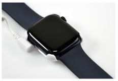
Pivot the other side of the wearable down into the tray sensor.
