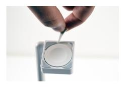
If using the charging cradle ZW1005, remove the top pad.
