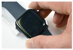
Press the 4 corners of the tray sensor against the wearable for at least 10 seconds.
