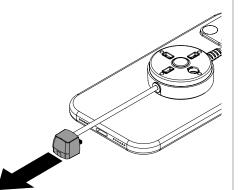
Insert the scraper removal tool (DNTX93) between the sensor and device. Carefully work the scraper tool back and forth to break the adhesive bond between the sensor and the device.
