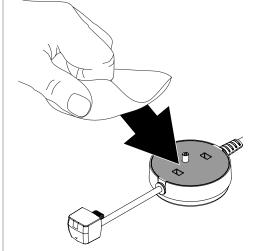
Remove one of the replacement adhesives (ADH2198) from it's backing and align it with the flat surface of the sensor. Smooth it into place for at least 10 seconds. **Note:** The sensor is now ready to be reinstalled. Consult the installation guide for more information.
