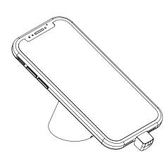
Lift the device and sensor from the stand and place a charged and coded OneKEY against the IR lens on stand. Press the button on the key to deactivate the stand.
