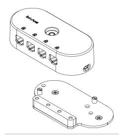
Use the provided alcohol wipe to clean the surface (above or below the counter) where the alarm unit will be placed. Allow it to dry completely.
