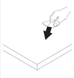
Pull the tab to activate the battery. The unit should make an audible "chirp".
