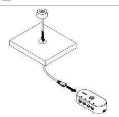
Peel the liner from the adhesive on the bottom of the IR dot.
