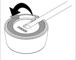
Place the IR dot in the desired location and apply pressure for at least 10 seconds.
