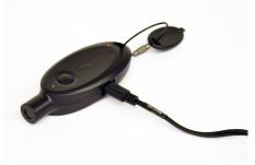
Allow the OneKEY to fully charge. The LED for the battery indicator will shine green when fully charged.
