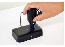
To program a OneKEY, place the Key into the port on the Programming Station. Press the button on the Key to transfer the code to the Key. It is now ready for use.
